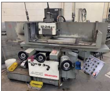
12" x 24" Okamoto ACC-12.24ST Surface Grinder
